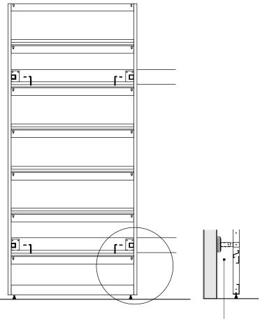
■ Distance between construction wall and wall-unit approx. 96mm by use of end-plate code 1022/235 or 1022/201 wirh width 146mm.
