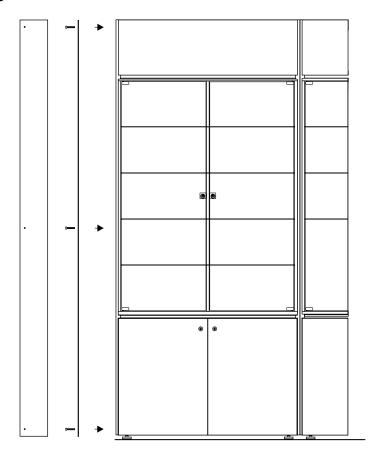
■ End-plates code 1022/235 or 1022/201 fixed to wall-unit with 3 bolts incl. nuts per end-plate.
